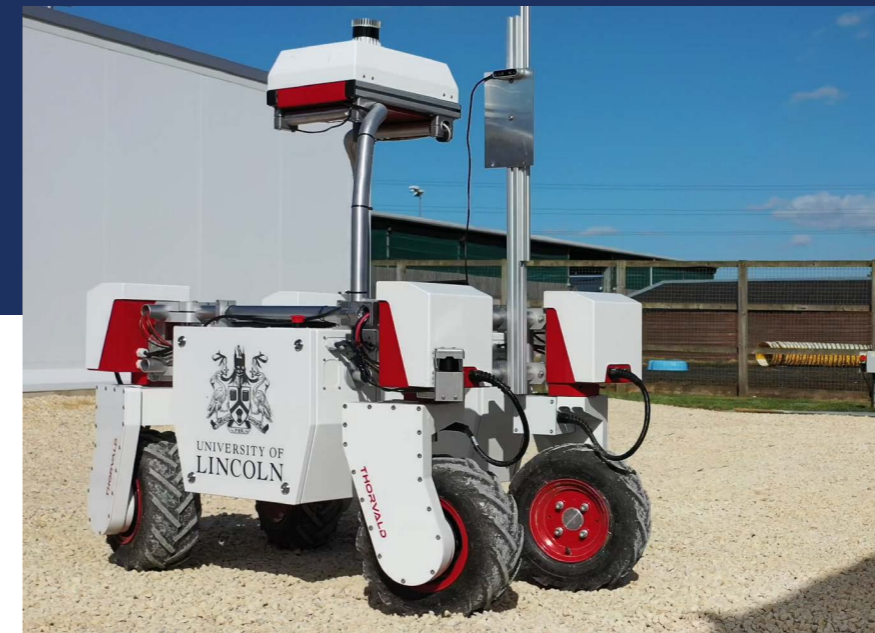
Thorvald is an advanced multi-functional autonomous platform supporting a number of LAR's agricultural projects.
